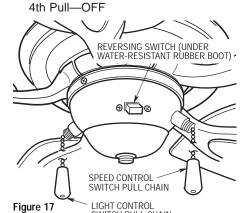
□3. If airflow is desired in the opposite direction, turn your fan off and wait for the blades to stop turning. Then slide the reversing switch (located under the rubber boot) to the opposite position (Figure 17), and turn the fan on again. The fan blades will turn in the opposite
